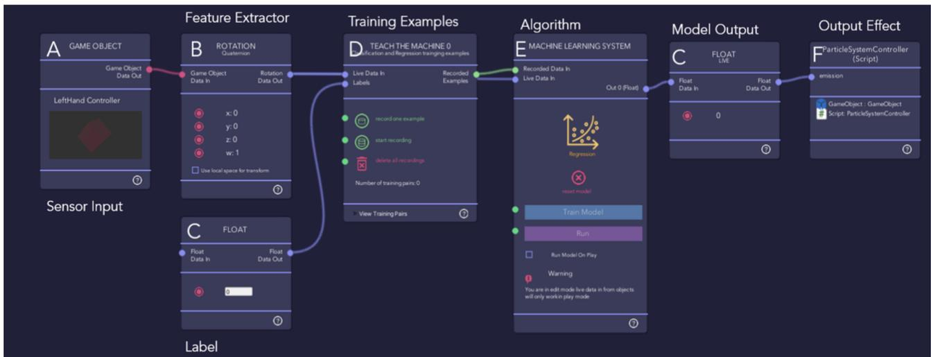
Figure 2: The InteractML node based scripting interface.
