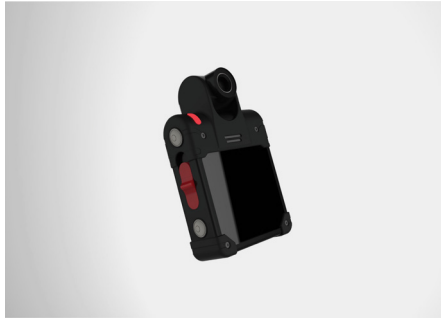
Figure 3 Three-dimensional render of alternative BWC with additional button
