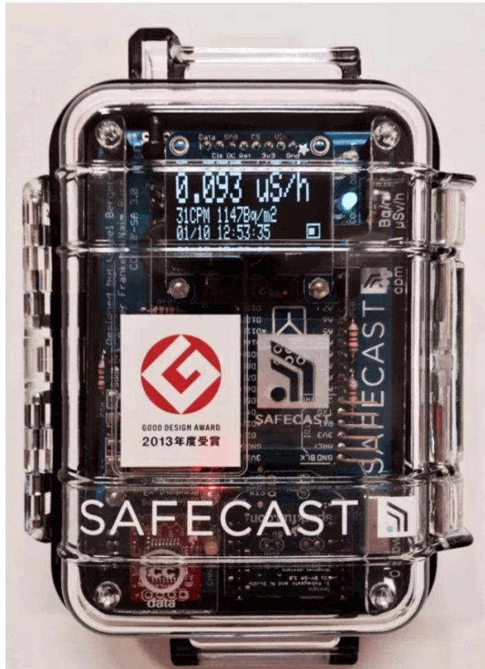
Figure 4.3: Safecast's bGeigie Nano. 334
