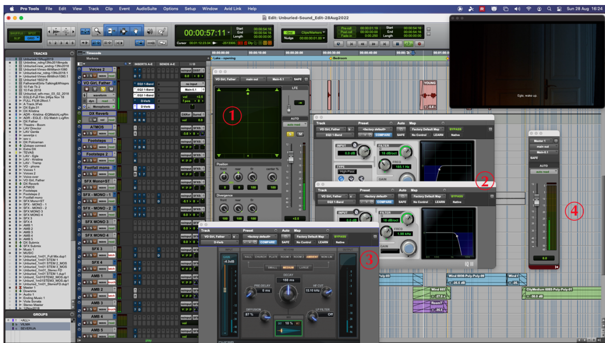
Fig. 3.3 Unburied : sonically embodying the voice of the ethereal girl: 1.the surround sound panner shows the mono audio of the original recording positioned exclusively in the centre channel; 2. the EG inserts roll off the low and high frequencies to create a muffled effect; 3. the reverb insert creates space around the voice, to position it in a physical interior; 4. the master fader shows that the audio of the girl’s voice comes solely through the centre channel.
