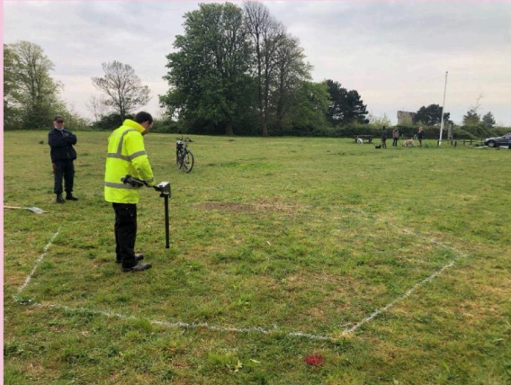
13 May 2021 Scanning for unexploded ordnance devices at Gunners Park, due to the site being on ex-MOD land (above) Breaking ground (below)
