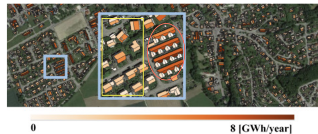
Fig. 2: Scattered houses solar potential(Yellow bounding box) and terraced houses overestimated solar potential(Red bounding circle) taken from [7]
