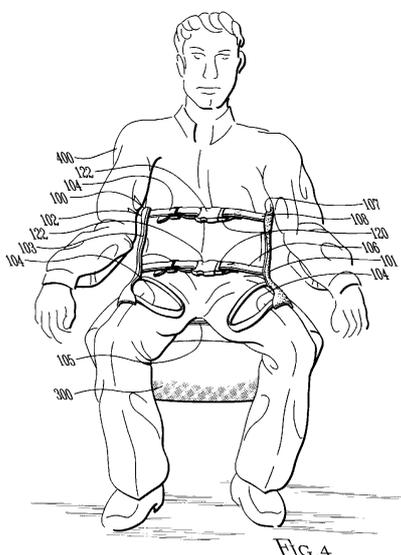
Figure 8 An illustration from a 1999 patent application showing a Tyvek harness for lifting passengers from an onboard wheelchair into their seat. Sling for transporting a person into a chair and method of using the same invented by Judy Hoit, US Patent 6276006B (Hickman, 2020)
