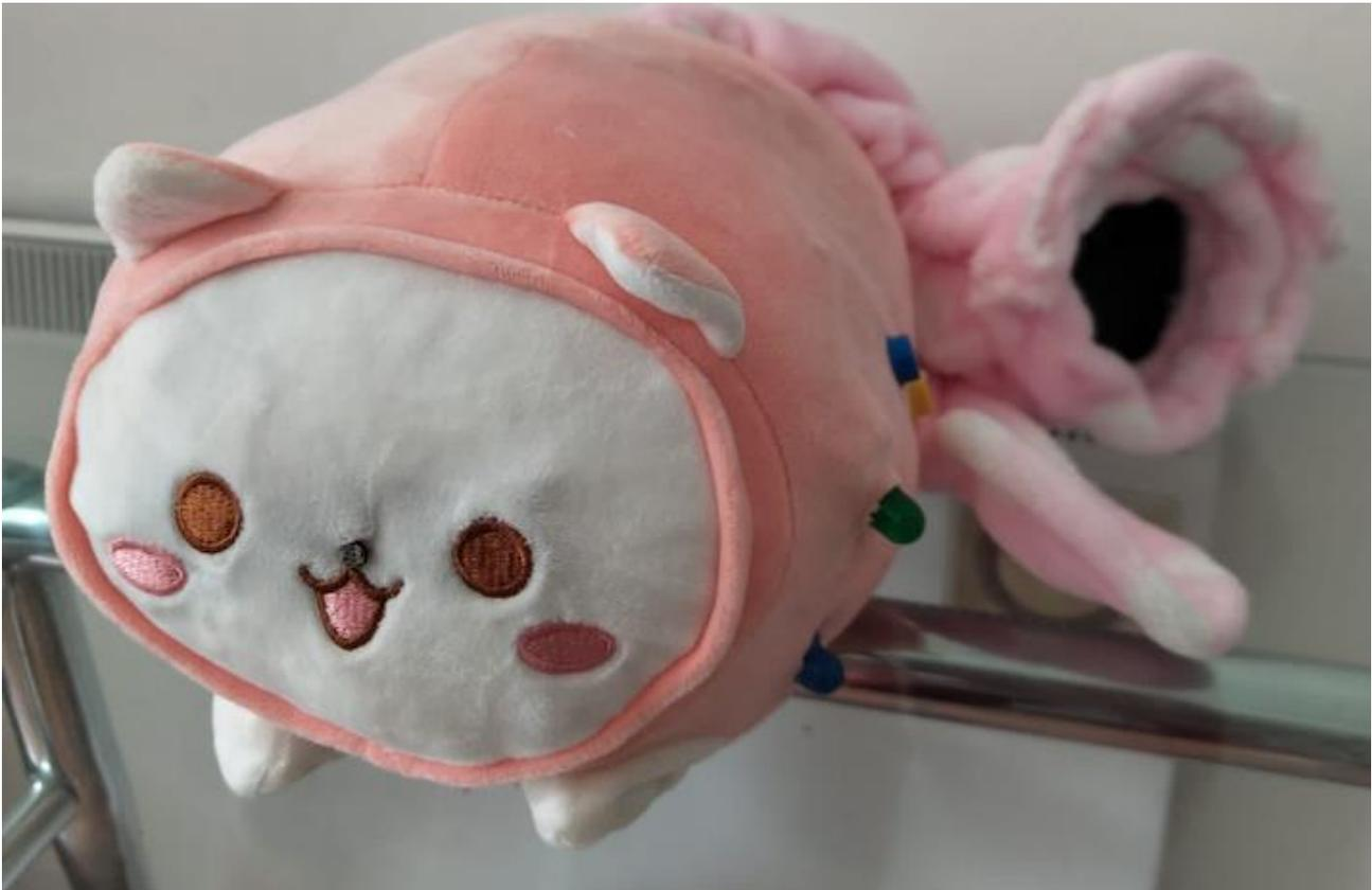
*Figure 79 The cat synth, SYNTHia showing the buttons, speaker and sensors embedded in the cat plushie.*
