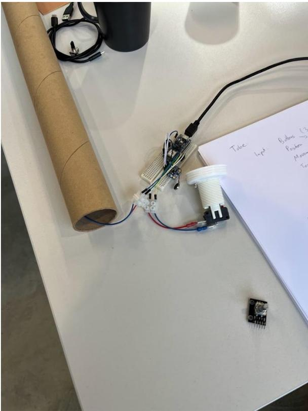
*Figure 71 Completed Rough Prototype including button installed in the top of a cardboard tube and circuit board with haptics attached.*
