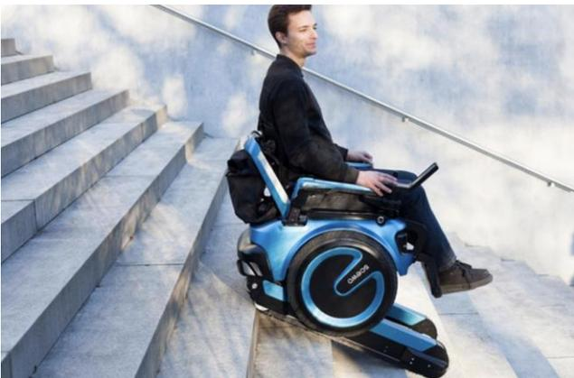
*Figure 9 The scewo is a self-balancing wheelchair that can go up and down stairs. (designboom, 2017)*
