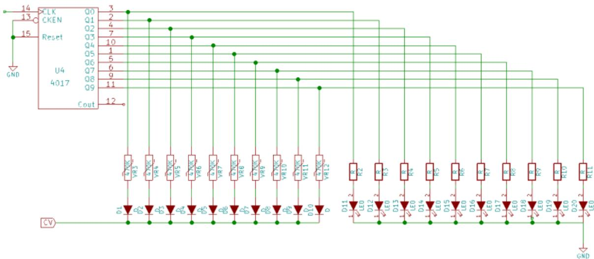
Figure 24 The Circuit Diagram for the Baby10 (Whiteford, 2016)
