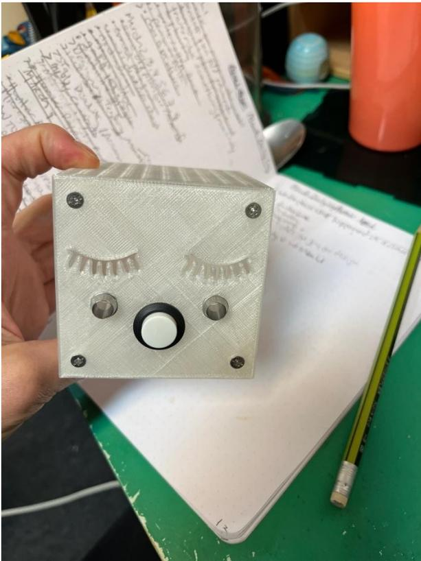
*Figure 69 Improved casing for version 4 showing inset screws.*
