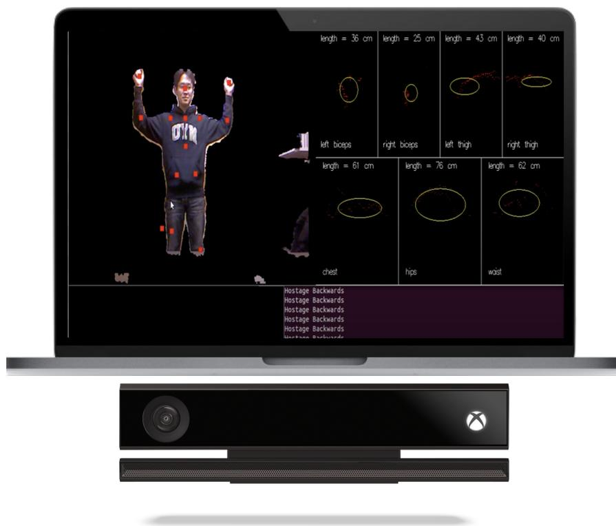
Fig. 4.8 demonstrates a mock-up of calculating human body segments from the Kinect sensors on the PC machine by [87]
