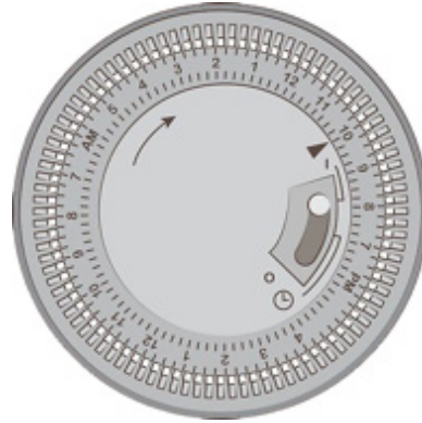
Figure 71. Mechanical timer switch interface.
