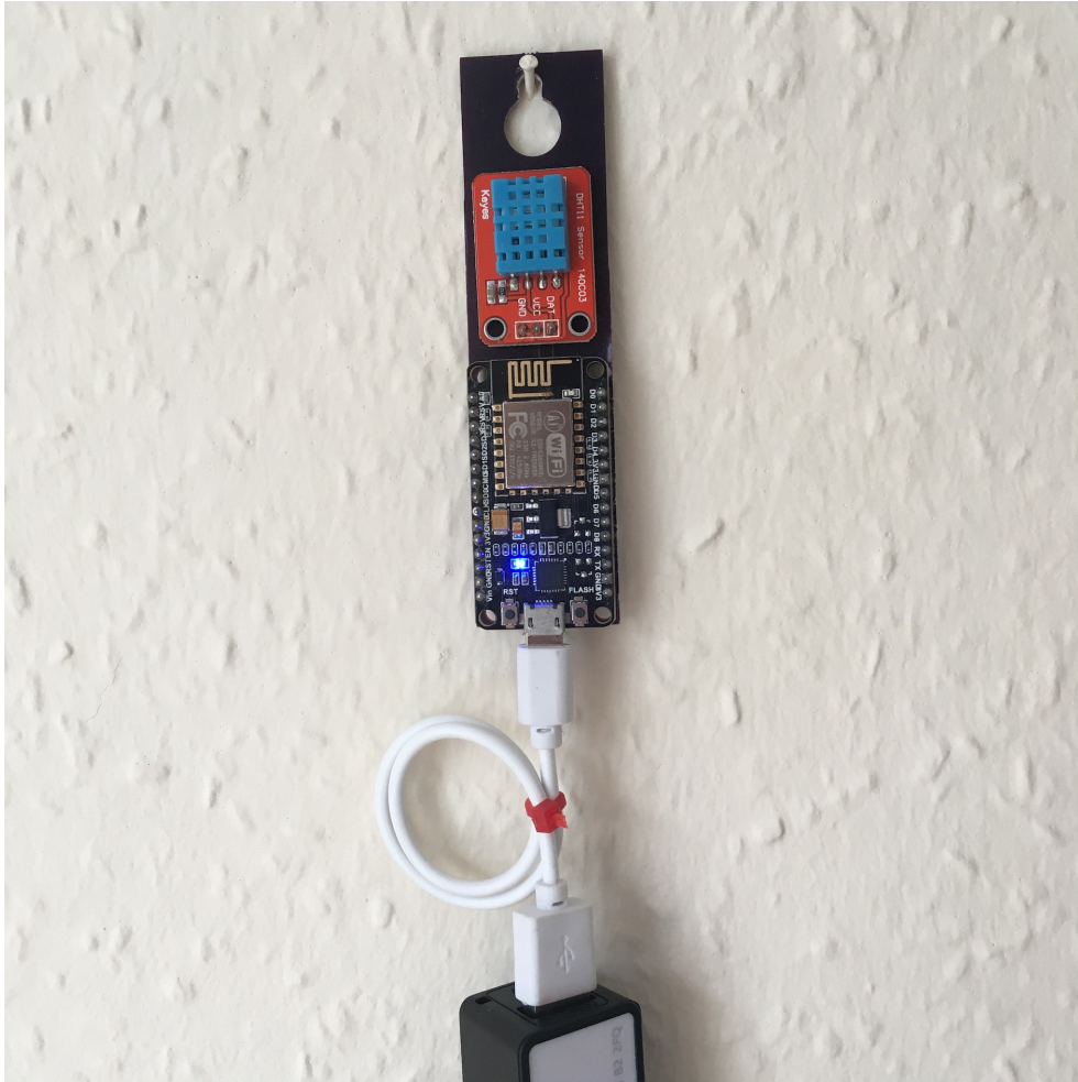
Figure 28. Humidity sensor (PCB version). © David Chatting.
