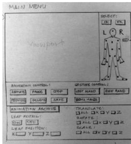
Figure 3.25: Initial sketches hand gesture interface design
