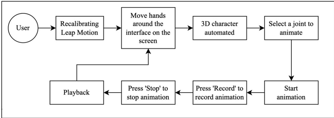
Figure 3.24: Hand gesture interface system design
