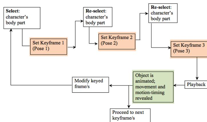
Figure 3.1: A typical process of keyframe animation
