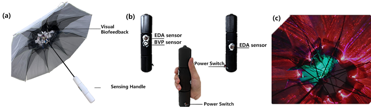
Figure 2: Affective Umbrella: sensing handle and visual biofeedback
