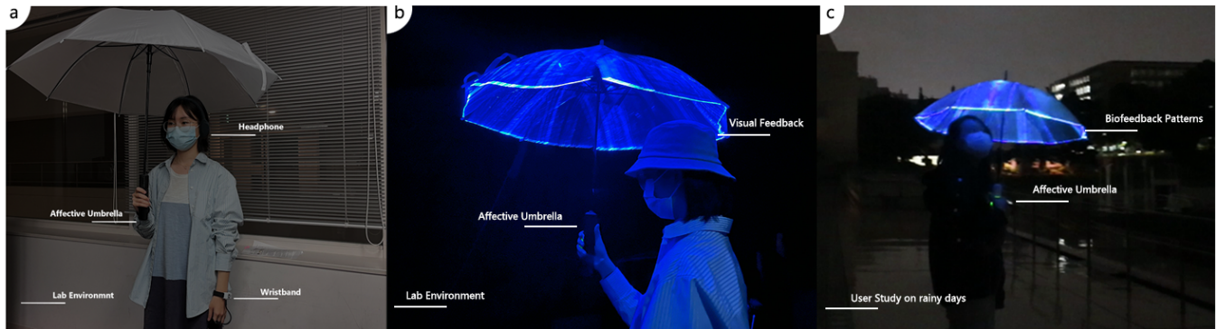
Figure 4: Design process in three phases. (a) Phase 1: User and umbrella, setup in the sensing test. (b) Phase 2: Umbrella in action in the feedback test. (c) Phase 3: Interaction use case; umbrella visualizes heart activity (light intensity change) and electrodermal activity (number of peaks influence the color) in the user study.
