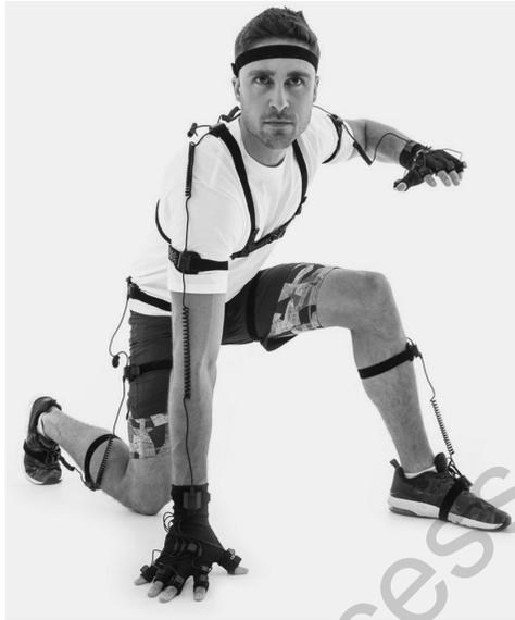
**Figure 11.6** The Perception Neuron motion capture system.
