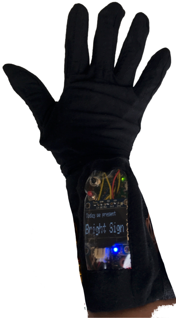
Figure 4.14: Updated glove design, with wearable sensors embedded in channels in an inner lining
