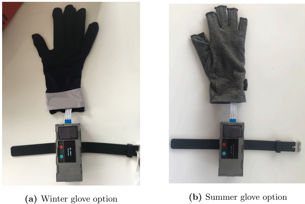
Figure 5.11: The assembled glove, flexible PCB and hard enclosure with a winter and summer textile option
