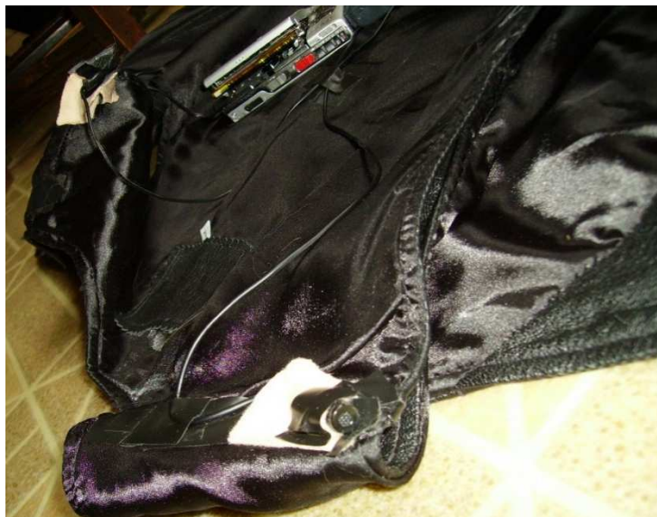
Figure 9 Shoulder-mounted microphone with Sony MZ-R50 MiniDisc recorder; recorder fits into an ordinary shirt pocket.
