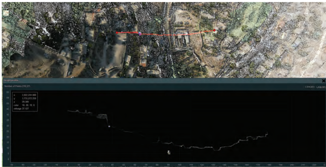
Figure 21. Using the Potree point cloud visualisation web interface a section can be visualised through the area of the Siloam pool where the first tunnel begins running under the Wadi Hilwe road.
