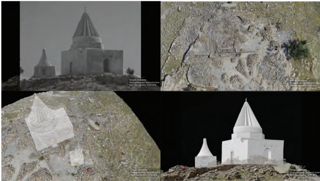
Figure 10: Series of Screenshots from Photogrammetry and reconstruction 3D modelling of the Amadeen Temple, Forensic Architecture. 2018
