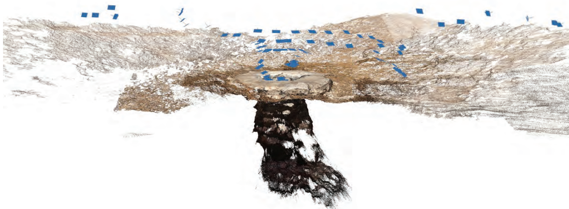
Figure 20: Point cloud of the well of Awimer Salman Abu Medigam, 2016. The blue rectangles depict the positions of individual image frames from which the 3D information was derived. Photo: Ariel Caine, Forensic Architecture, 2017
