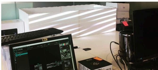
It is controlled with the same middleware software than the actual facility and driven by MAC laptop with two Triple Head to go, Matrox graphics cards, providing a complete canvas resolution of 7680 x 800 pixels and frame rate of 60 Hz.
