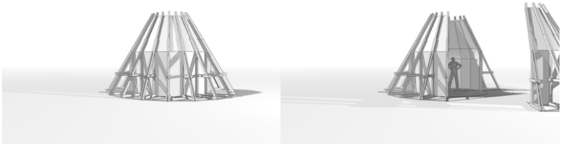
Fig. 4.08, 4.09 - assemblage in circle and in half-circle
