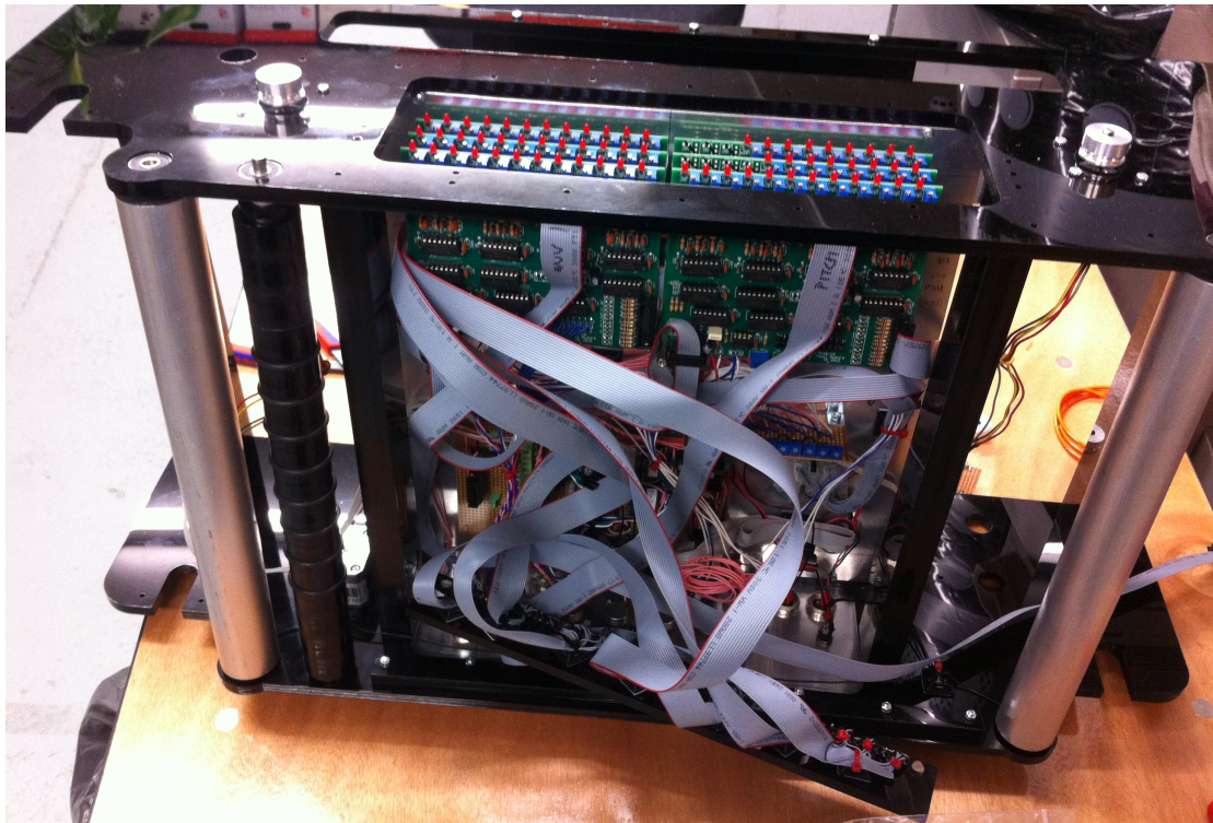
Fig. 43. Attaching the numerous ribbon cables from the light sensors or 'play head' to the graphic input modules. March 2016
