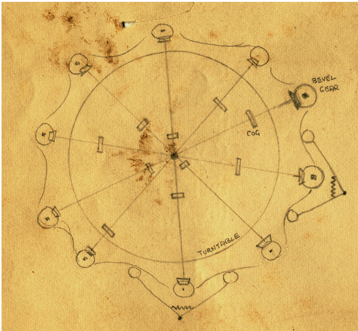
Fig. 10a: Daphne Oram's diagram for a radial tape-drive system (detail).
