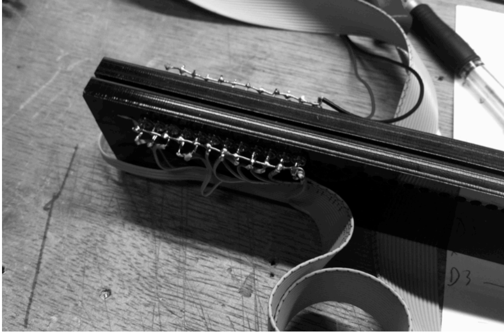
Fig. 35. Wiring the pitch parameter's light sensing components using ribbon cable in order to test the control circuitry.
