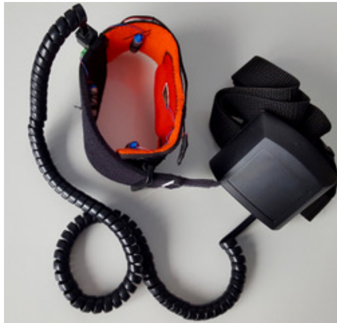
Figure 1. The VARM system: module box (on the right), coiled cabling and the Velcro strap with four motors attached.
