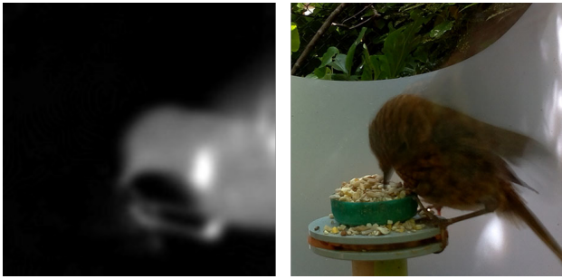
Figure 4: A ‘difference image’ (left) triggers image capture a moment later (right) when contiguous areas of change are within a minimum and maximum threshold.
