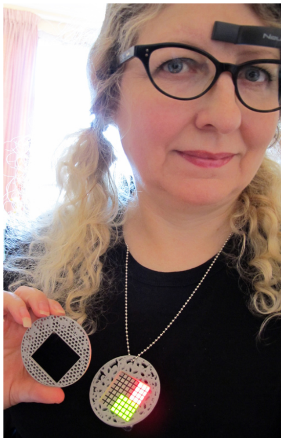
FIGURE 4.10: EEG Visualising Pendant showing live EEG data sent from a MindWave Mobile Bluetooth headset. The pendant is shown featuring one of a number of interchangeable 3D printed alumide frames (2013)
