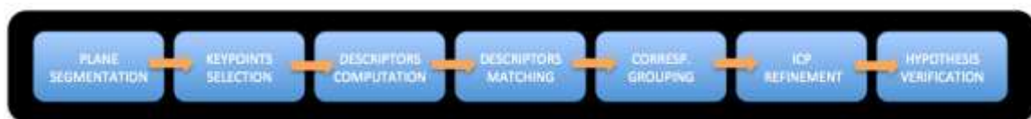
Fig.3. The recognition and pose estimation algorithm pipeline.
