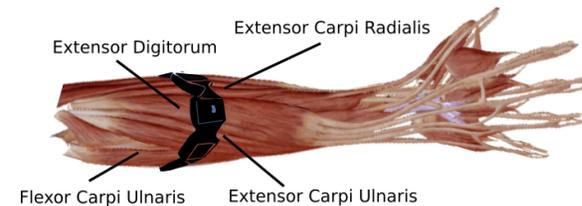
**Figure 1:** Position of the device on the forearm.
