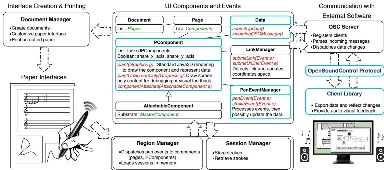
**Figure 4: PaperComposer programming API supports creation of paper interfaces to manipulate musical data. Developers edit blue elements to identify data types, specify data representations and define user interactions.**
