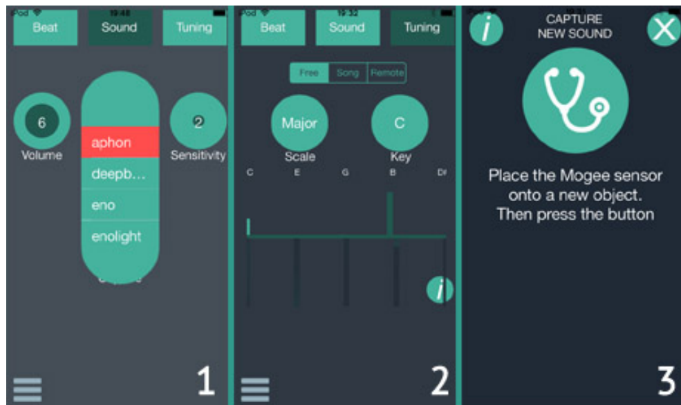
Figure 4.9: The graphical interface of the Mogeess software application: the sound view (1), the tuning view (2) and the capture view (3).
