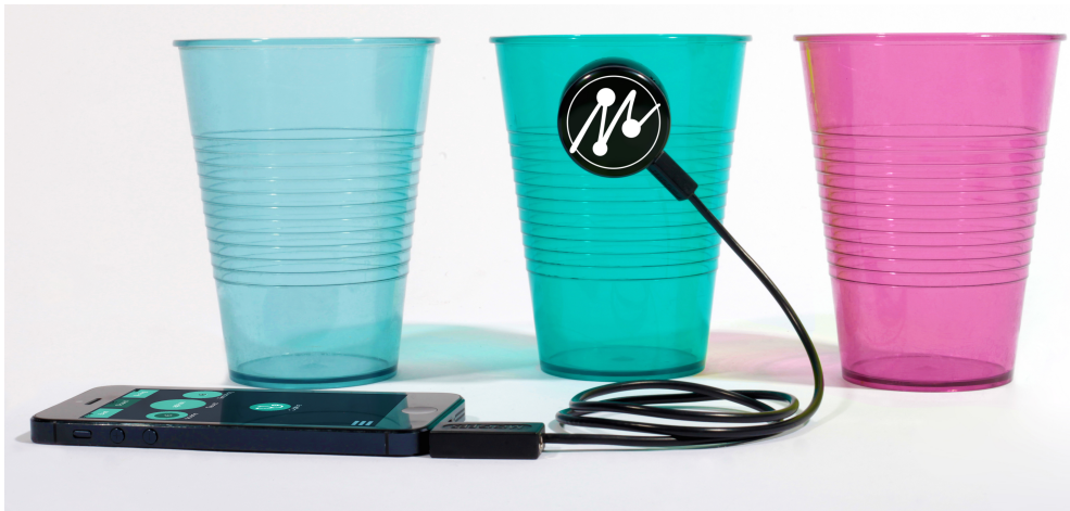
Figure 4.8: A typical usage of the system: the hardware unit is connected to an iPhone through a cable and attached to a resonant object (a plastic glass).
