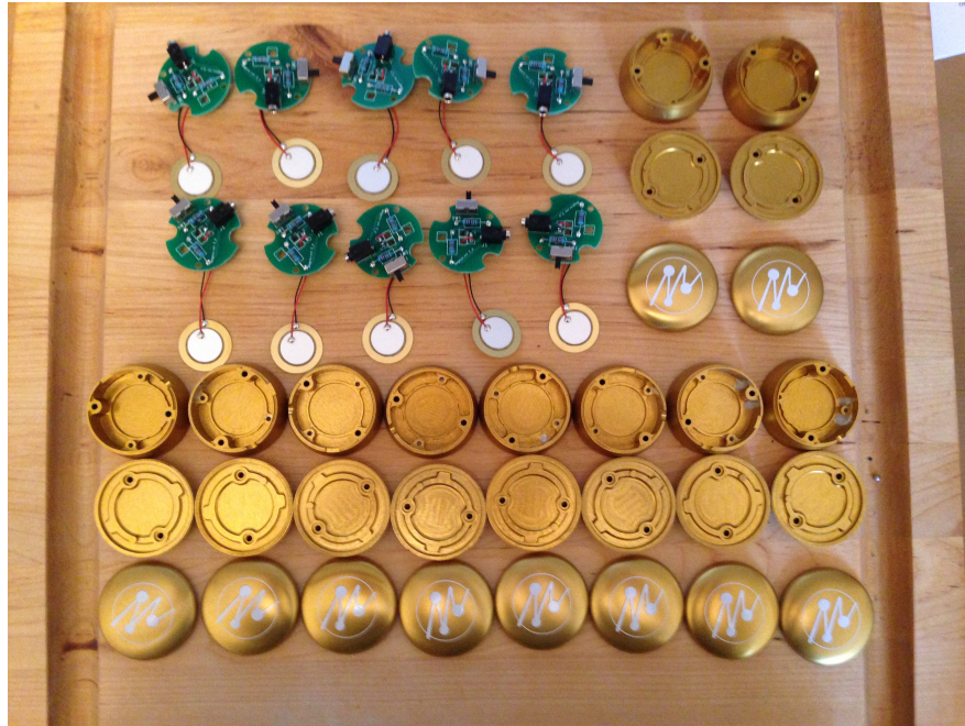
Figure 4.10: Components of the Mogeas hardware unit, consisting in a piezo-transducer sensor, a printed circuit board and an aluminium case.
