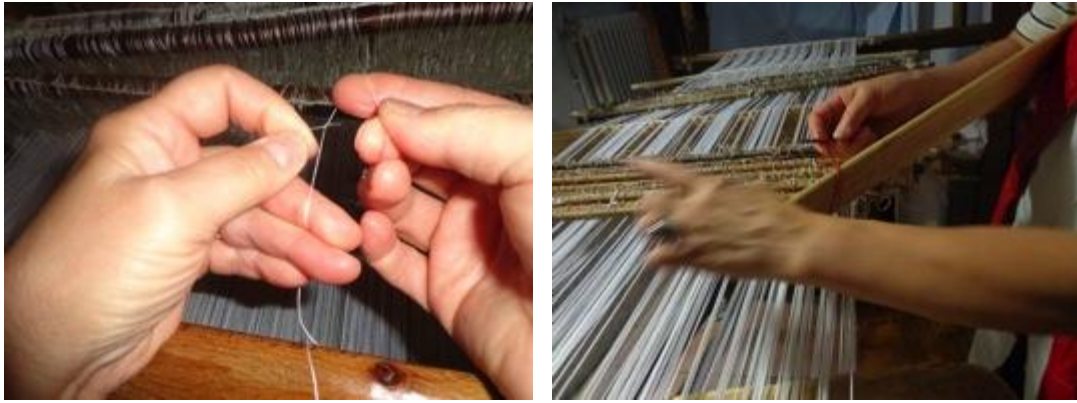
Fig. 6.5 Weaver's knot, Maria showing me how to tackle mistakes (left)
