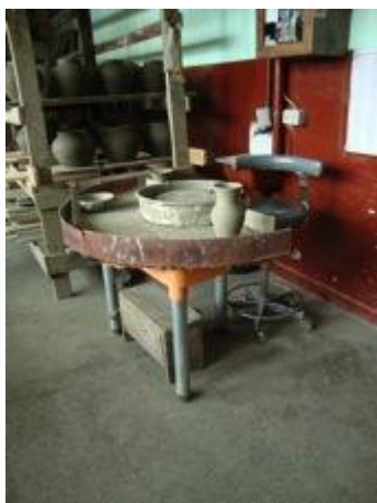
Fig. 8.11 Modern Canadian electric wheel used to produce traditional black pottery (left).
