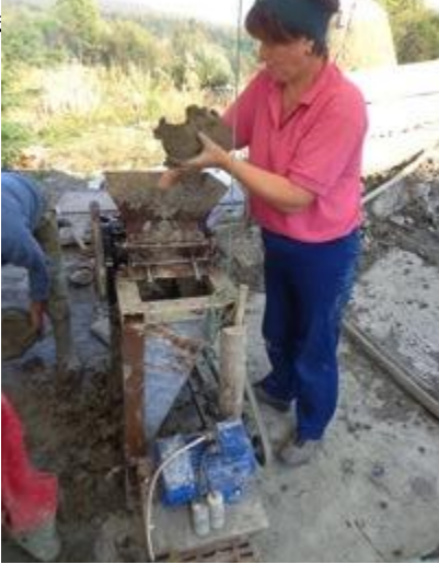
Fig.7.10 Mixing the clay in the malaxor (left)
