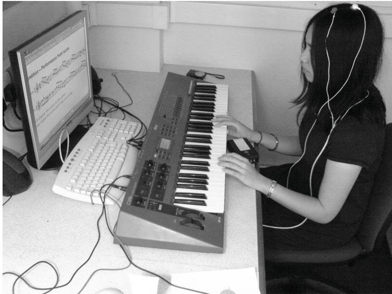
Figure 5.1: Photo of the experimental setup showing the EEG amplifier connected wirelessly to a laptop, and MIDI keyboard connected to a computer which also showed the experimental stimuli
