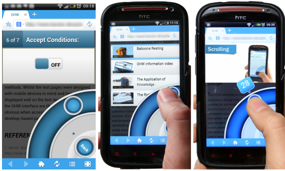
Figure 3: A checkbox input rendered by the OHW, where a tap on the OHW interface toggles the state (left), a user selecting a video from the media menu (middle) and video playback control (right).
